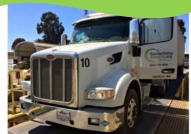
This grant purchased two new fuel-efficient transfer trucks that utilize compressed natural gas (CNG) engines resulting in cleaner air emissions from approximately 72,000 miles of on-road miles per year, producing 90% lower NOx emissions than EPA standards. The new transfer trucks replaced two older diesel engines that have taken place of circulation.
